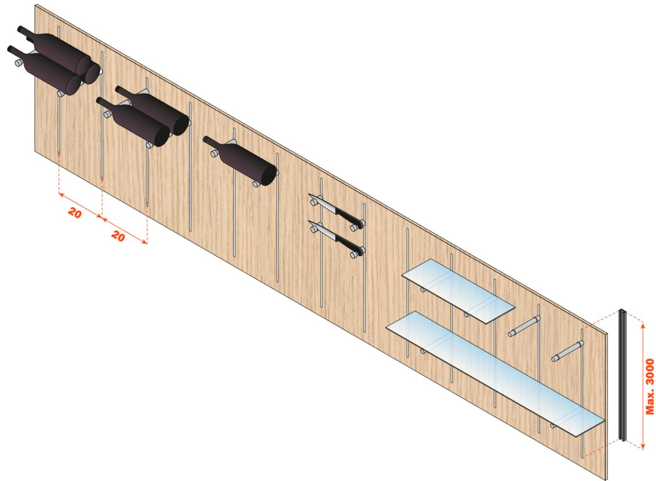
When machining the wood panel, leave 100 mm from the top and from the bottom of the panel.
