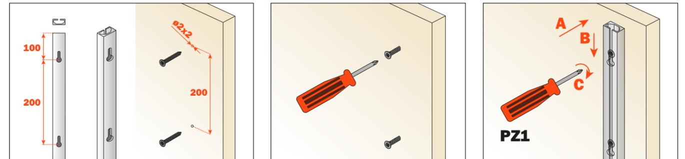
Drilling the wood panel to fix the surface-mounted profile. Use the screws supplied with wall plugs.
