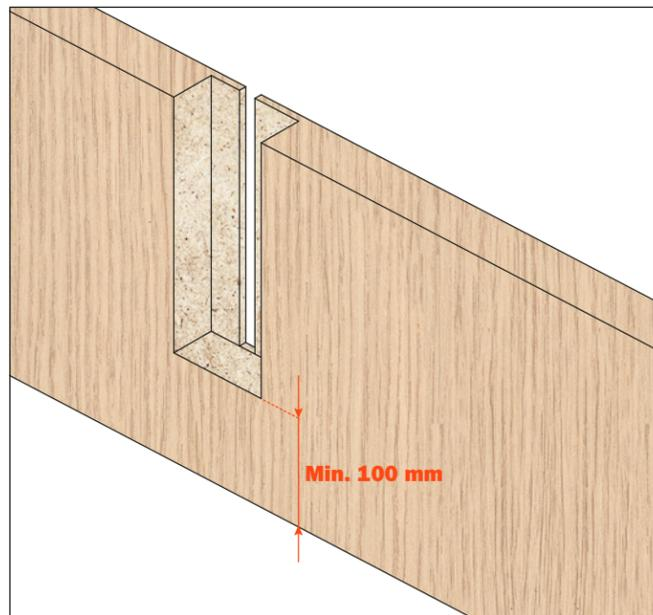
Dimensions for machining the panel.
